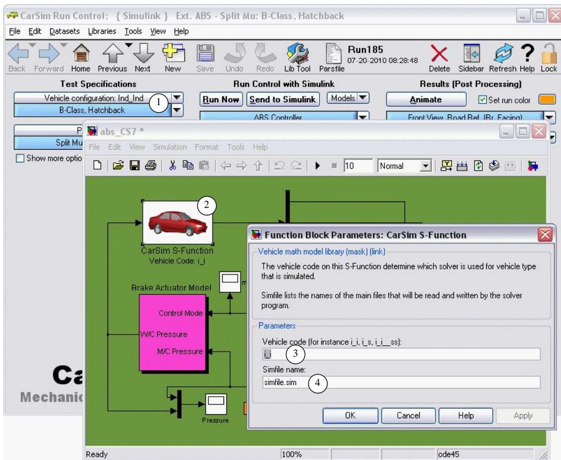
Figure 2. Simulink model with one VS vehicle model.
