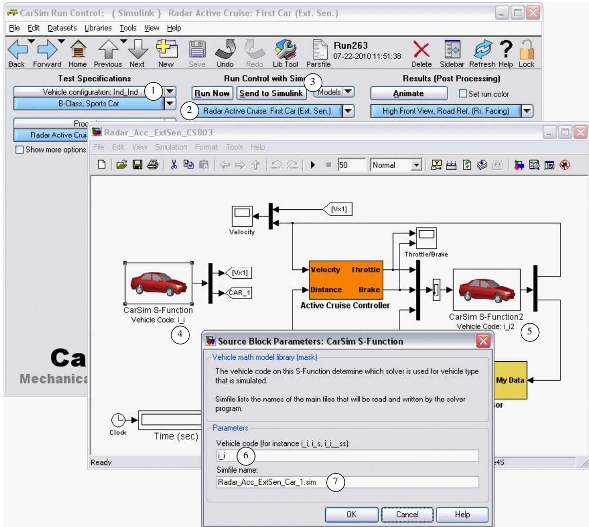
Figure 3. Example Simulink model with two vehicles that interact.
